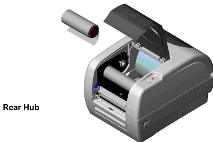
Fig. 5 Ribbon installation (II)
