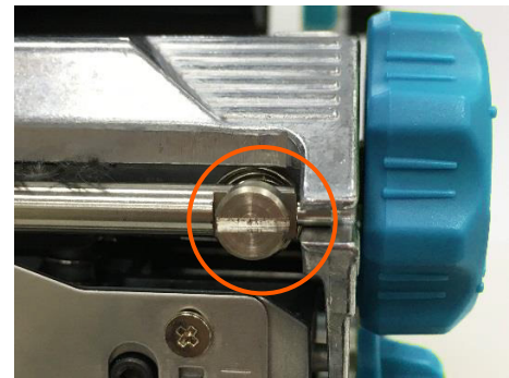
Ribbon tension adjustment knob
